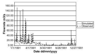
Fig. 3 Comparison of observed and SWAT daily flows for 1991, calibration period 1989 to 1994
